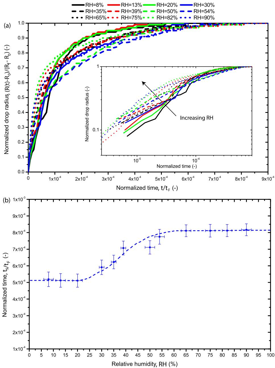
**Fig. 7.** (a) Normalized drop radius,  $(R(t) - R_0)/(R_f - R_0)$ , as a function of normalized time,  $t/t_F$ , for different humidities, and (b) Normalized total time of spreading,  $t_s/t_F$ , as a function of RH. The inset graph is a log-log representation for all RH values.
