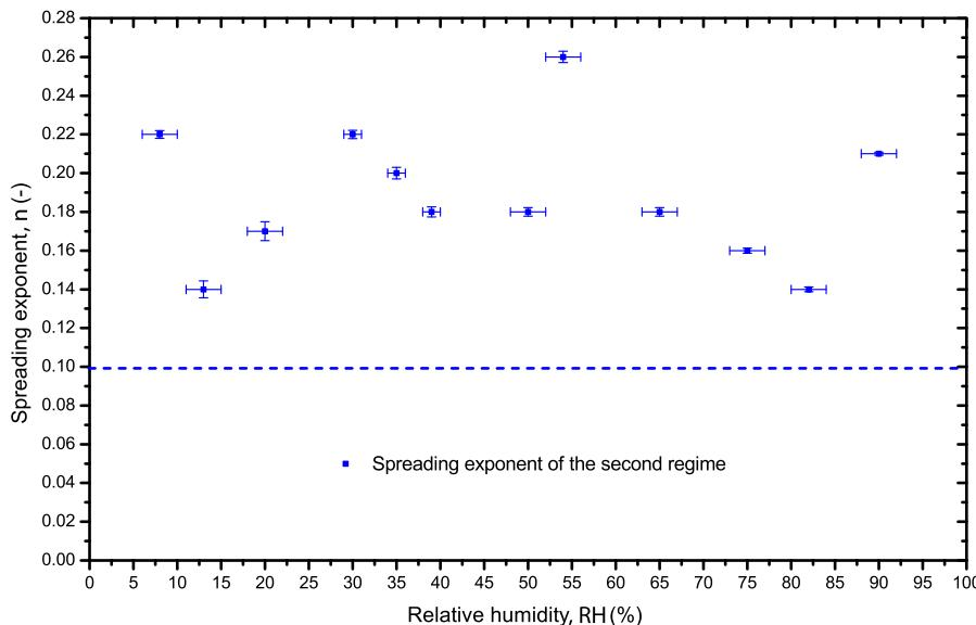
**Fig. 11.** Spreading exponent of the second regime of spreading (mean value  $\bar{n} = 0.19 \pm 0.04$ ) compared to the spreading exponent of Tanner's model ( $n=0.10$ ) as a function of the RH.
