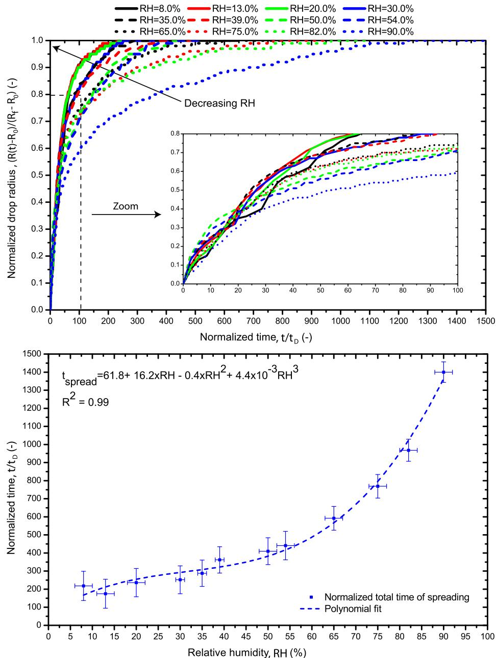
**Fig. 8.** (a) Normalized drop radius,  $(R(t) - R_0)/(R_f - R_0)$ , as a function of normalized time,  $t/t_D$ , for RH varying from 8% to 90%. The inset graph is a magnification of  $t/t_D$  from 0 to 100. (b) Normalized total time of spreading,  $t_s/t_D$ , as a function of RH.
