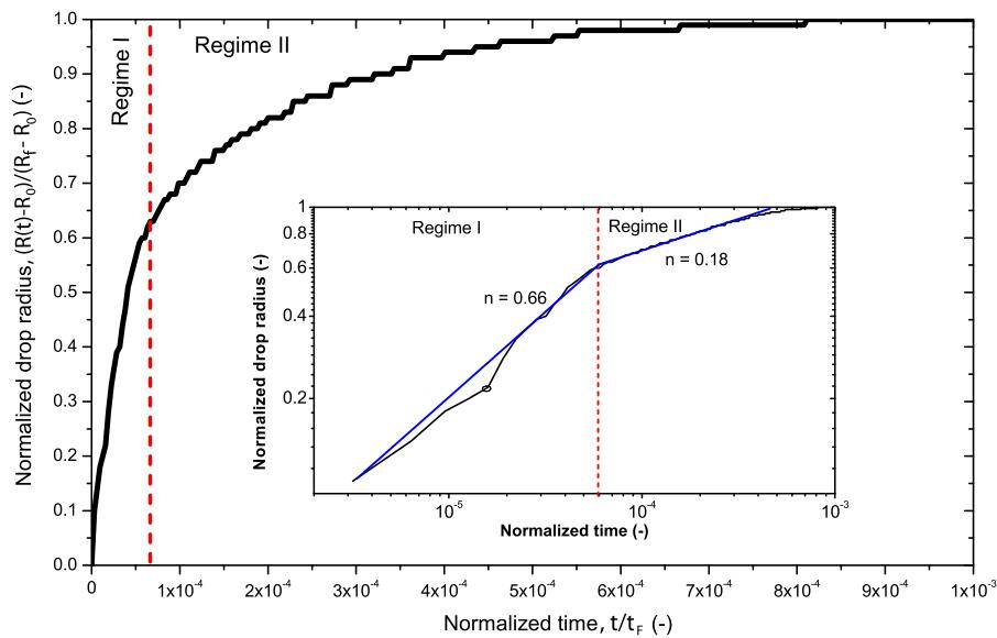
**Fig. 4.** Evolution of the dimensionless radius,  $(R(t) - R_0)/(R_f - R_0)$ , as a function of dimensionless time,  $t/t_F$ , at RH = 65%. The inset graph is a plot in a log-log representation.
