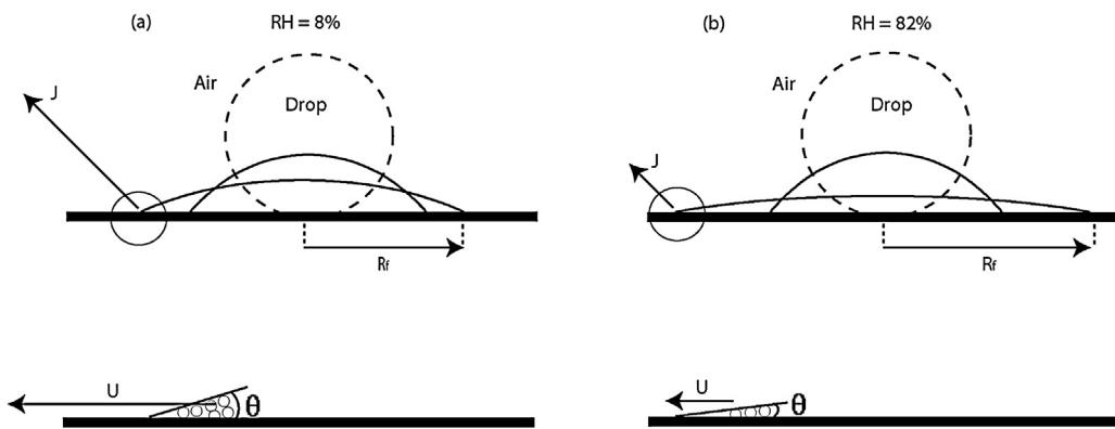
**Fig. 9.** Schematic representation of spreading drops for the case of: (a) RH = 10% and (b) RH = 80%. Initially, the blood drop has a spherical shape, and at equilibrium the drop has the shape of a spherical cap. The arrows indicate the velocity and evaporative flux of water vapour from the drop surface to the surroundings in the vicinity of the triple line. The dashed square marks the area close to the triple line, where the drop geometry can be approximated by a wedge.
