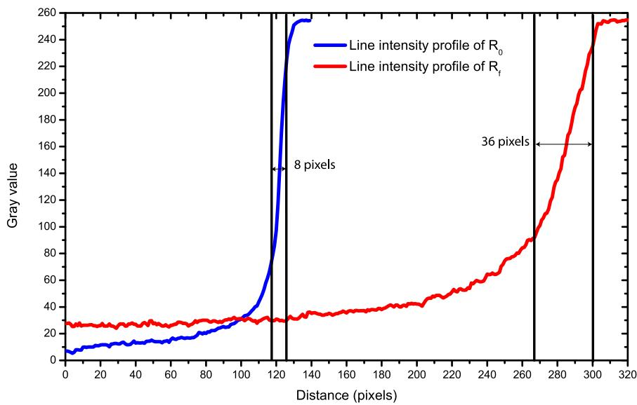
**Fig. 2.** Intensity along the straight line of an initial deposited radius  $R_0$  and of a final wetted radius  $R_f$ . The bars given in the plot show that the measured uncertainty of  $R_f$  is higher than that of  $R_0$ .
