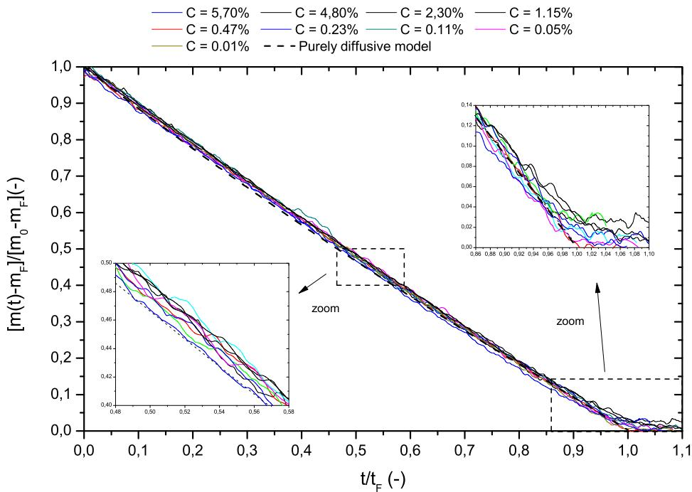
**Fig. 6.** Normalized mass variation as a function of normalized time for nanofluid concentrations ranging from 0.01% to 5.70% (room humidity of 50%). The inset is a magnification of  $t/t_D$  from 0.85 to 1.10 that illustrates the effect of the concentration on the final stage of drying. The dashed line is Eq. (2).
