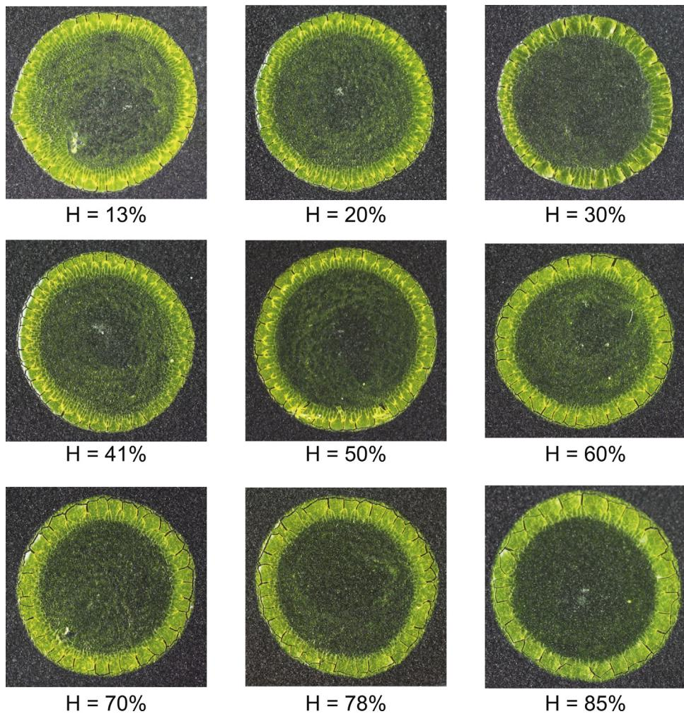
**Fig. 8.** Influence of humidity ranging from 15 to 87% on pattern formation (nanofluid concentration of 1.15%).
