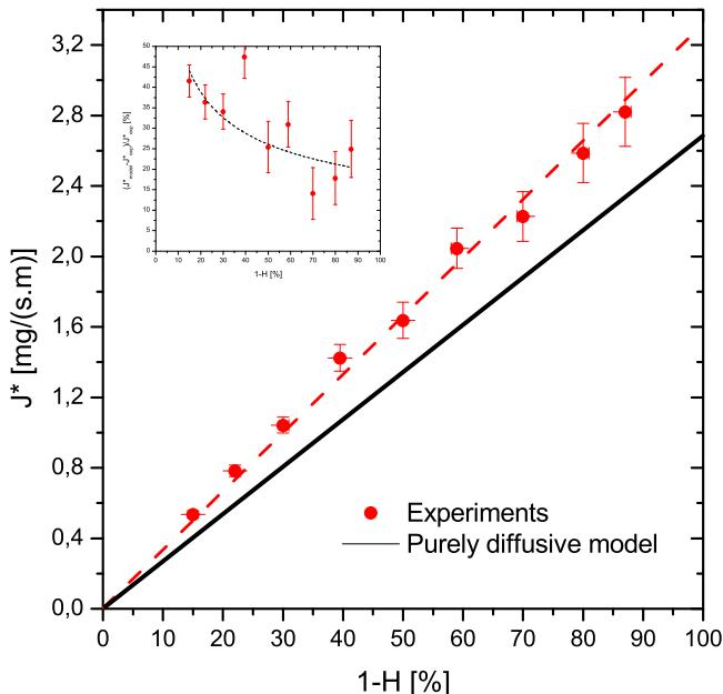
**Fig. 9.** Evaporation mass flow rate per drop radius as a function of the  $[1 - H]$  for the same nanofluids with a concentration of 1.15%. The experimental results were compared to those of a purely diffusive model based on Eq. (2). Linear evolution of both  $J^*$  with  $J^* = \alpha(1 - H)$  with  $\alpha_{\text{exp}} = 3297 \text{ mg s}^{-1} \text{ m}^{-1} \pm 1.35\%$  and  $\alpha_{\text{model}} = 2664 \text{ mg s}^{-1} \text{ m}^{-1} \pm 1.27\%$ .
