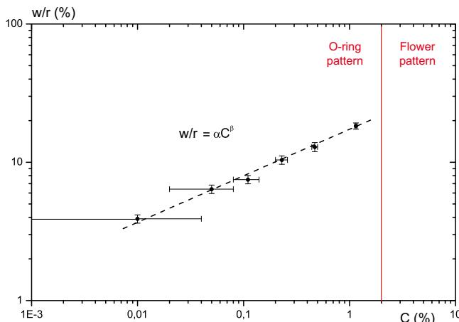
**Fig. 7.** Dimensionless o-ring width [ $w/r$ ] as a function of the nanofluid concentration (constant room humidity of 50%).  $w/r = \alpha C^\beta$  with  $\alpha = 1.72 \pm 1.92\%$  and  $\beta = 0.346 \pm 4.23\%$ .
