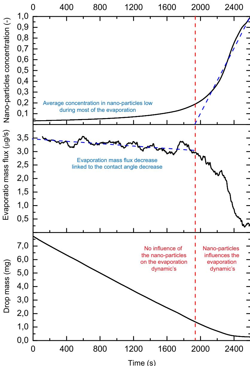
**Fig. 3.** Mass evolution (bottom figure), evaporation mass flux (middle figure) and mean solid concentration (top figure) as a function of time for a nanofluid concentration of 4.8% at a room humidity of 50%. Two stages of evaporation can be noticed depending on the mass flow rate of evaporation: one when the evaporation mass flux decreases linearly and the other when the evaporation mass flux sharply decrease.
