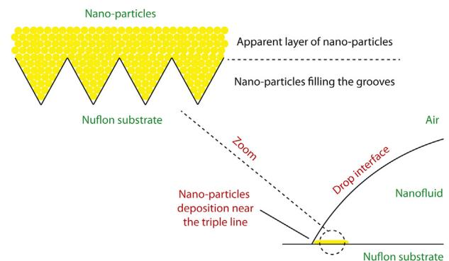
Fig. 4. Nano-particle deposition in substrate grooves.
