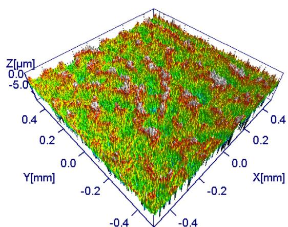
**Fig. 2.** Surface roughness using a confocal microscope (STILL Micromesure 2). Average standard roughness of 1.736 µm.
