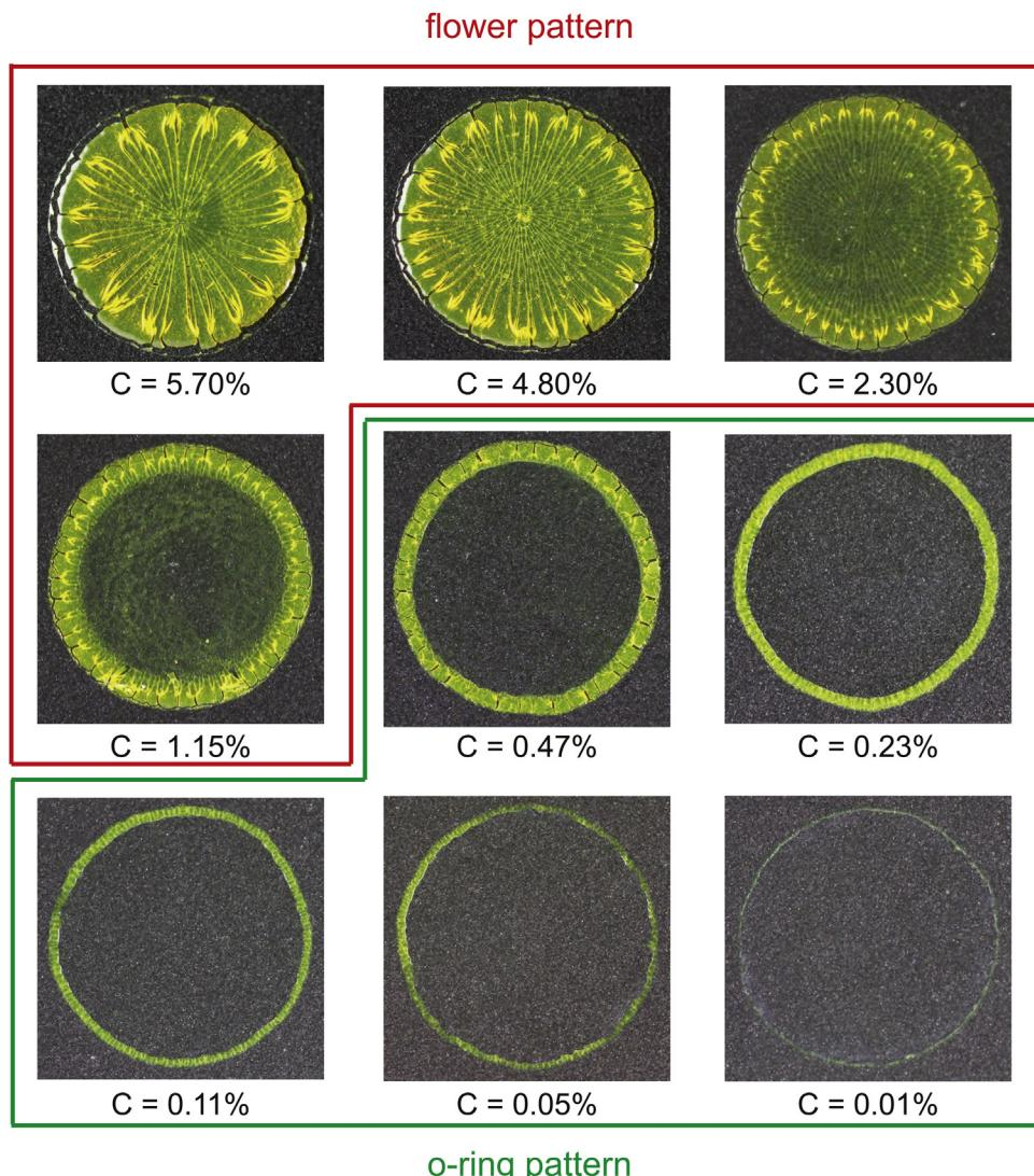
**Fig. 5.** Influence of nanofluid concentrations ranging from 0.01% to 5.70% on pattern formation (glovebox humidity of 50%, room temperature of  $25.0^\circ\text{C} \pm 0.6^\circ\text{C}$ ).
